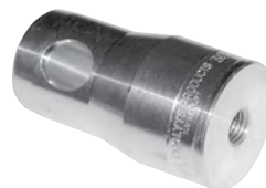
CCS7-702/12 weight = 0,265 kg Offset half conical coupler Offset 31 mm, thread M12
