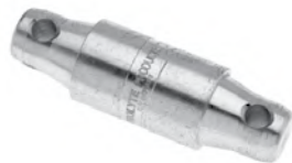
CCS4-S05 through CCS4-S50 weight = 0,070 - 0,170 kg Spacers X = 5 mm to 50 mm in steps of 5 mm
