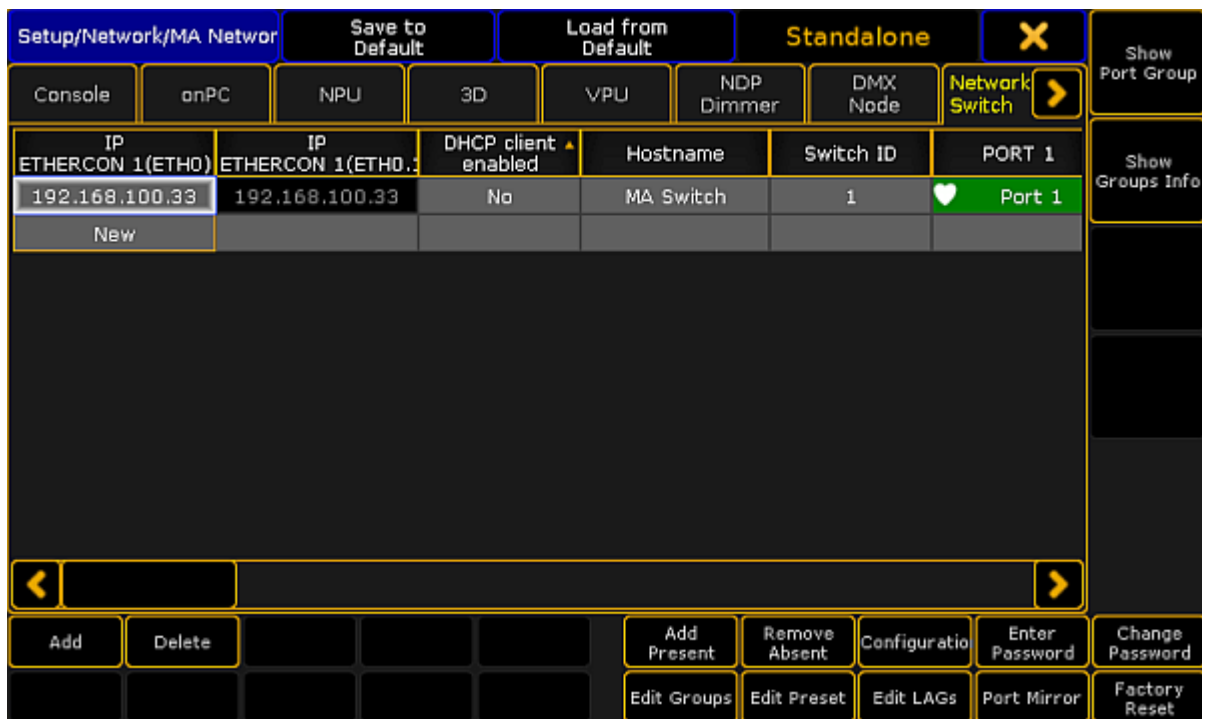
MA Network Configuration - Network Switch
