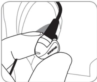
Insert the earphones so they form a tight seal. The fit of the earphone can greatly affect sound quality.
