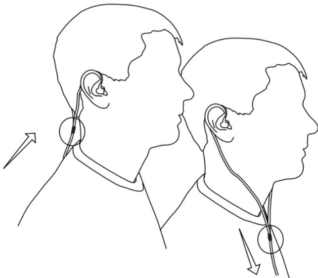
Wearing the cable over the ear and securing it behind the head can help keep the earphones in place during physical activity
