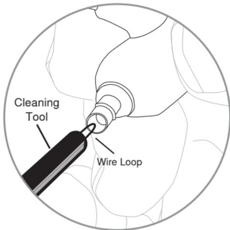
**Caution:** When cleaning, do not force any object through the earphone nozzle! This will damage the earphone sound filter.
