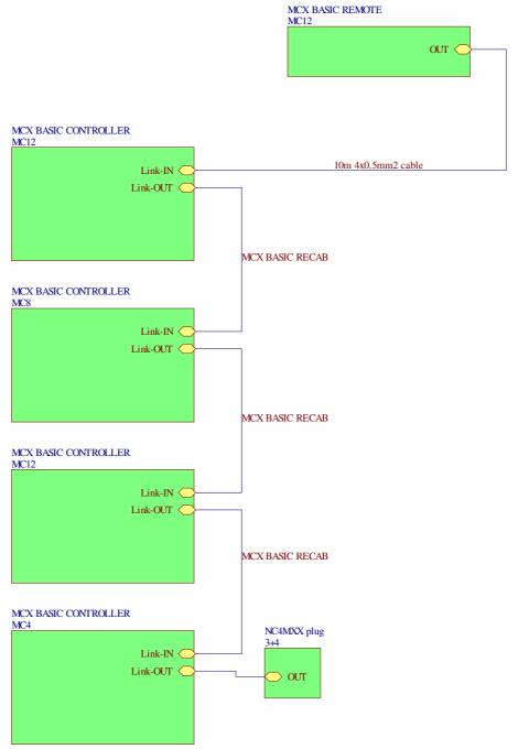
During operation, the NC4MXX plug must be connected to the last controller in chain
