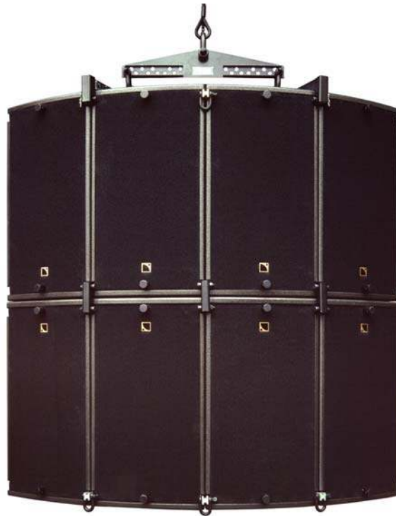
8 ARCS Enclosures providing 90 degree horizontal coverage and +40/-40 degree vertical coverage (coupled double row configuration)
