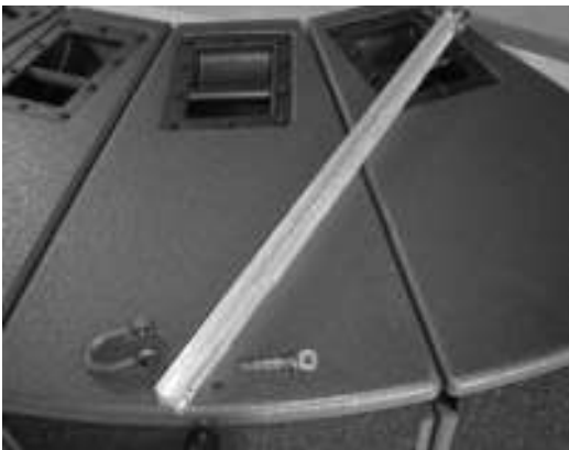
(5) Front shackle removed from ARCOUPL
