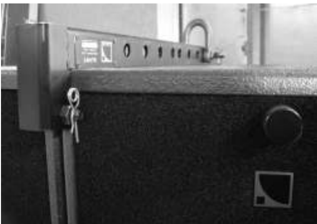
(13) Front locking nut and bolt assembly installed with safety, pick point selected on BUMP3
