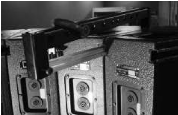
(7) BUMP3 slides into position from the rear
