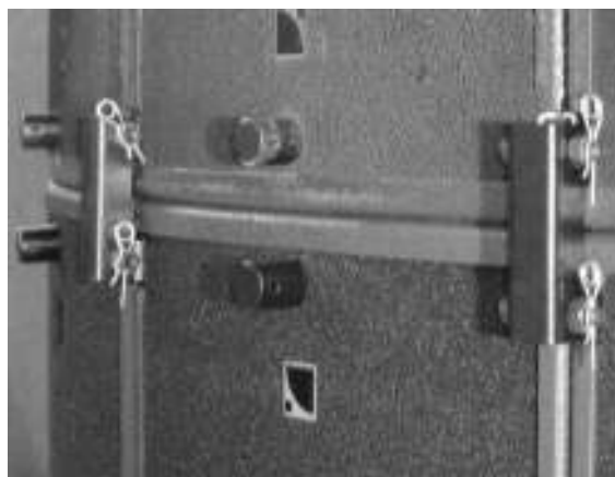
(4) ARCSTRAP secured using a locking nut and bolt assembly with cotter pin safety
