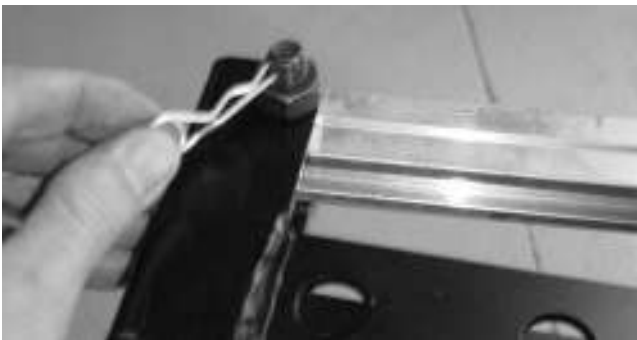
(11) ARCOUPL secured using a locking nut and bolt assembly with cotter pin safety
