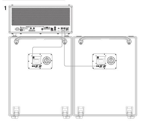
In example 1 above, a speaker cable with 1/4" ends connects from one speaker output of the amplifier to the speaker input of the Ampeg SVT-410HE cabinet. An additional cabinet may be connected by attaching another speaker cable from the remaining 1/4" speaker output of the amplifier to a speaker input of the next cabinet.
