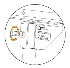
2. Remove the bracket from the enclosure.
