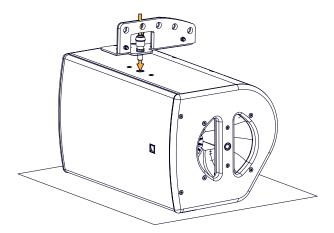
3. Rotate the X-BAR until perpendicular to the front grill.
