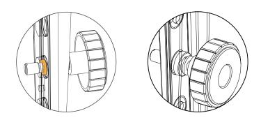
**4.** Tighten the knobs and fly the enclosure with a clamp.
