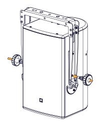
Make sure the safety washer goes through the hole on the bracket.
