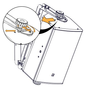
**3.** Remove the U-bracket and X-UTILT from the wall.
