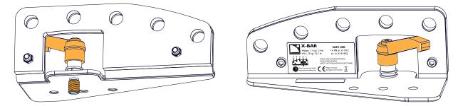
X-BAR shall be secured to the inserts on the enclosure, perpendicular to the front.
