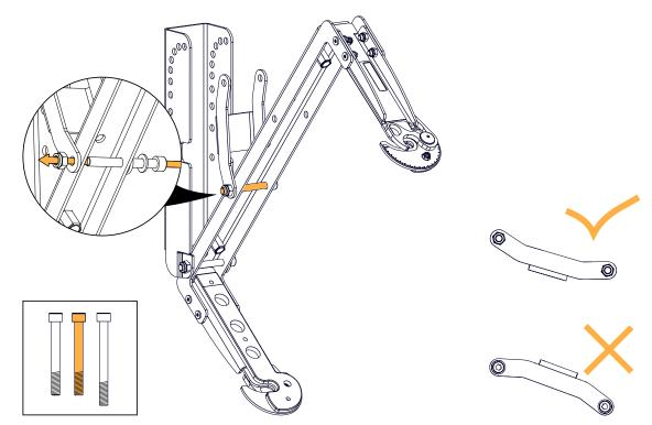
**4.** Choose the site angle and secure the rigging arm to X-UTILT. Refer to the angles on the label.
