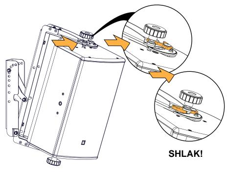
8. Set the azimuth angle.
