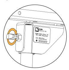
5. Loosen the knobs to set the site angle.
