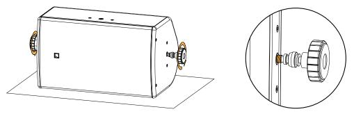
**6.** Lift the enclosure by the knobs and place it inside the U-bracket.
