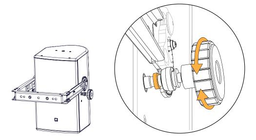
**3.** Push down until the knobs are locked inside the spring-lock mechanism.
