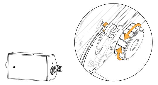
4. Push until the knobs are locked inside the spring-lock safety mechanism.
