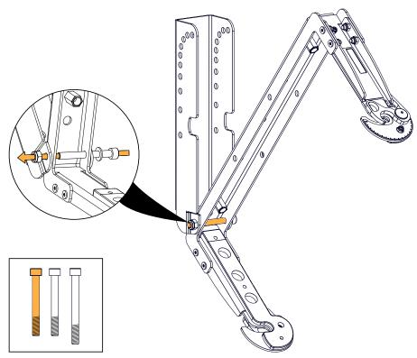
**3.** Secure the rigging arm to the U-bracket.
