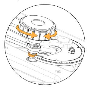
7. Push until the knobs are locked inside the spring-lock safety mechanism.
