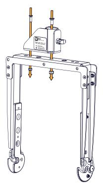
2. Secure the U-bracket to the enclosure using the additional holes.
