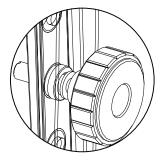
3. Tighten the knobs, reverse the assembly and mount it on a pole.
