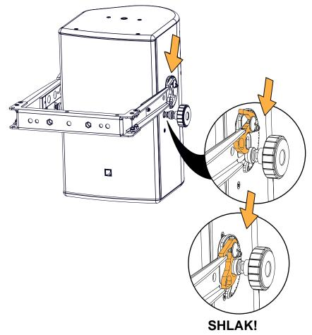
Alternatively, use the additional hole on the U-bracket.
