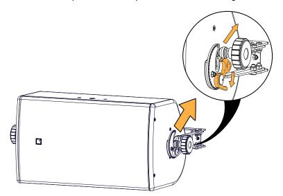
**3.** Remove the U-bracket from the wall.
