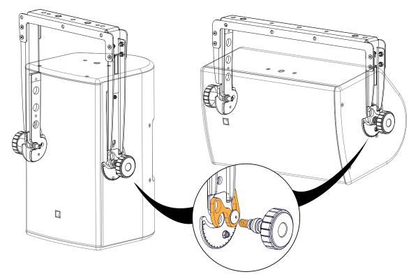
The threaded knobs feature a washer as a safety to avoid the accidental loosening of the knob.
