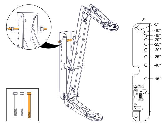
Drive the knobs in the inserts on the enclosure.
