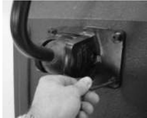
(2) Attach Omnimount plate to enclosure
