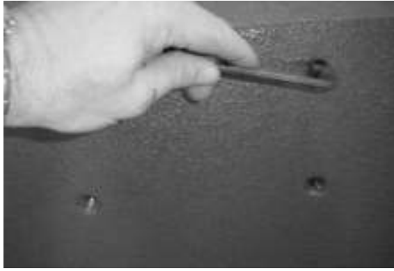
(1) Remove Omnimount attachment screws (5 mm allen key)
