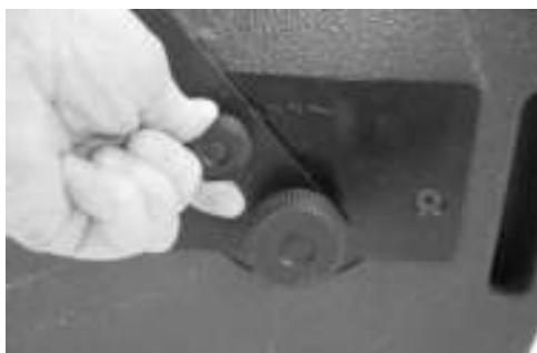
(9) The smaller knob allows for tilt angle adjustment
