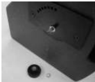
(7) Remove ETRI attachment knob and lock washer
